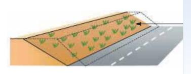
In areas where sufficient land is available, slope re-grading may be carried out, as part of a road widening scheme, to ensure stability. Re-graded slopes quickly vegetate and may even be hydro-seeded to assist in stabilising the slope and for visual effect. The stability of the cutting is improved but the geological interest is obscured.
